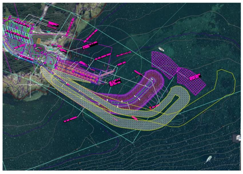
Yellow outline – original Burbury rock wall alignment Purple – Option 1 RFI submitted rock wall alignment and land-based infrastructure Yellow – Option 2 Extended rock wall alignment (excluding land-based infrastructure shown on this diagram)
